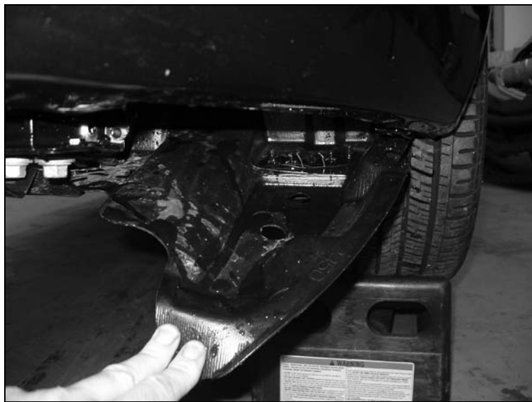
Figure 5. Gain access to the rear of the vent grille opening by pulling the wheel well cover down.
